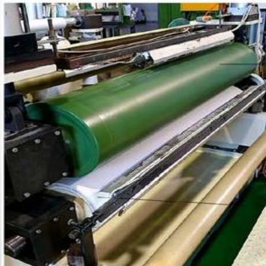
Hard Hot roller 2-layer iron roller with Teflon coating
